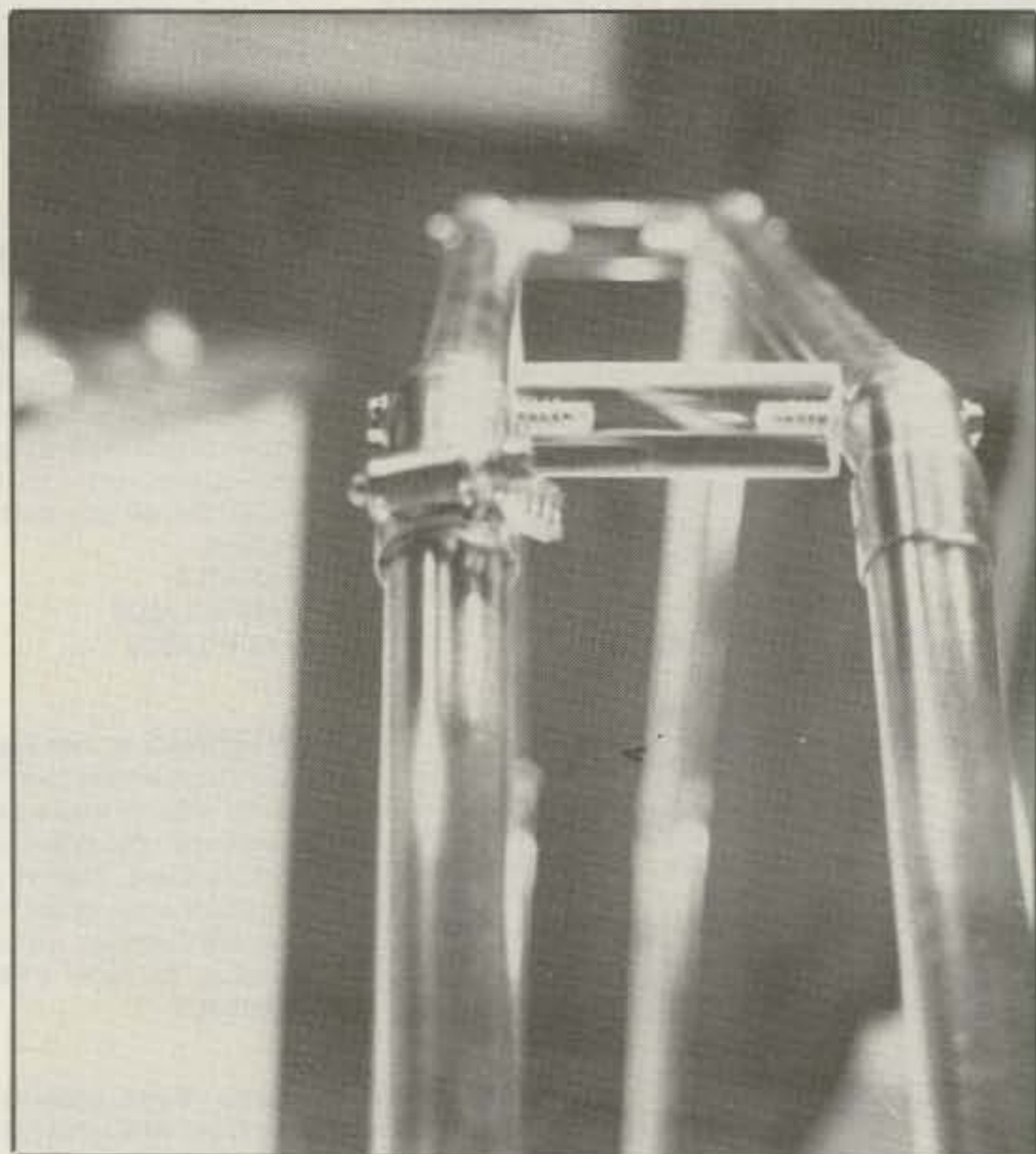
Fig. 4— The Plexiglass rods between the two turns of the loop are held in place by self-tapping screws through holes in the pipe.
